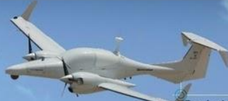
Dominator UAV Aeronautics Operational Altitude: 30,000 feet Wingspan: 13.5m Endurance: 28h
