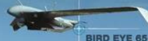
BIRD EYE 650 IAI Operational Altitude: 3,000 feet Wingspan: 3m Max Payload Weight: 1.2Kg Endurance: 3h
