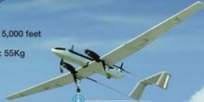
Panther IAI Operational Altitude: 5,000 feet Wingspan: 8m Max Payload Weight: 10Kg Endurance: 6h
