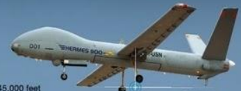
Hermes 900 Elbit Operational Altitude: 33,000 feet Wingspan: 15m Max Payload Weight: 300Kg Endurance: 40h
