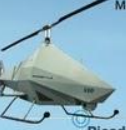
Picador VTOL UAV Aeronautics Operational Altitude: 12,000 feet Max Payload Weight: 180Kg Endurance: 8h
