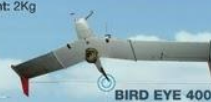
BIRD EYE 400 IAI Operational Altitude: 1,000 feet Wingspan: 2.2m Max Payload Weight: 1.2Kg Endurance: 1h
