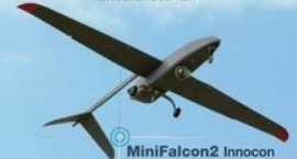
MiniFalcon 2 Innocon Operational Altitude: 18,000 feet MTOW: 150kg Wingspan: 5.5 meter Endurance: <15 hours Max. Payload weight: <35kg
