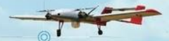
Mini Panther IAI Operational Altitude: 2,000 feet Wingspan: 2.5-3.5m Max Payload Weight: 2Kg Endurance: 1.5h
