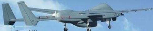
Heron 1 IAI Operational Altitude: 30,000 feet Wingspan: 16.6m Max Payload Weight: 250Kg Endurance: 45h
