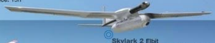
Skylark 2 Elbit Operational Altitude: 5,000-15,000 feet Wingspan: 6.5m Max Payload Weight: 9Kg Endurance: 4h
