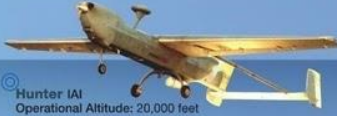
Hunter IAI Operational Altitude: 20,000 feet Wingspan: 10.5m Max Payload Weight: 100Kg Endurance: 21h
