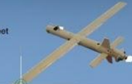
Sparrow UVision Operational Altitude: 10,000 feet Wingspan: 2.4m Max Payload Weight: 12Kg Endurance: 7h
