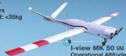
I-view MK 50 IAI Operational Altitude: 15,000 feet Wingspan: 5.3m Max Payload Weight: 10Kg Endurance: 6h
