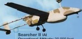
Searcher II IAI Operational Altitude: 20,000 feet Wingspan: 8.55m Max Payload Weight: 100Kg Endurance: 15h
