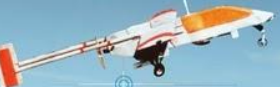
Pioneer IAI Operational Altitude: 4,600 feet Wingspan: 5.2m Max Payload Weight: 35Kg Endurance: 5h
