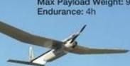
Skylark 1LE Elbit Operational Altitude: 500-15,000 feet Wingspan: 2.9m Max Payload Weight: 990g Endurance: 3h
