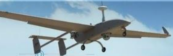
Aerostar UAV Aeronautics Operational Altitude: 18,000 feet Wingspan: 7.5m Max Payload Weight: 50Kg Endurance: 12h
